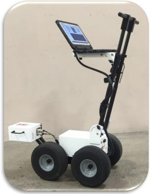
▲ Rugged, Portable Hardware ▲ ▲ Configurable Sampling Interval (1"/25mm default) ▲ ▲ Laser Option for Pavement Texture ▲
